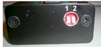
Figure 2 DIP switches and advance curve selection.
